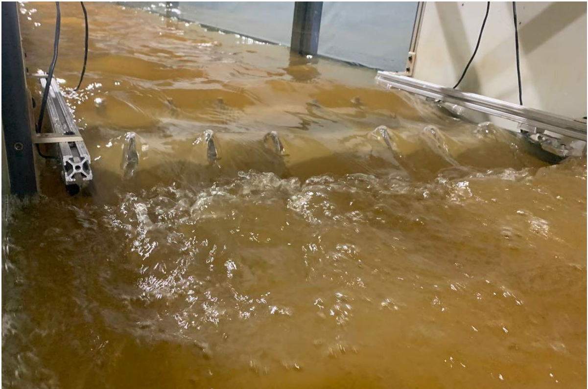
Figure 4.1 Small-scale bridge testbed during a running flow experiment to see inundation depth effect.
